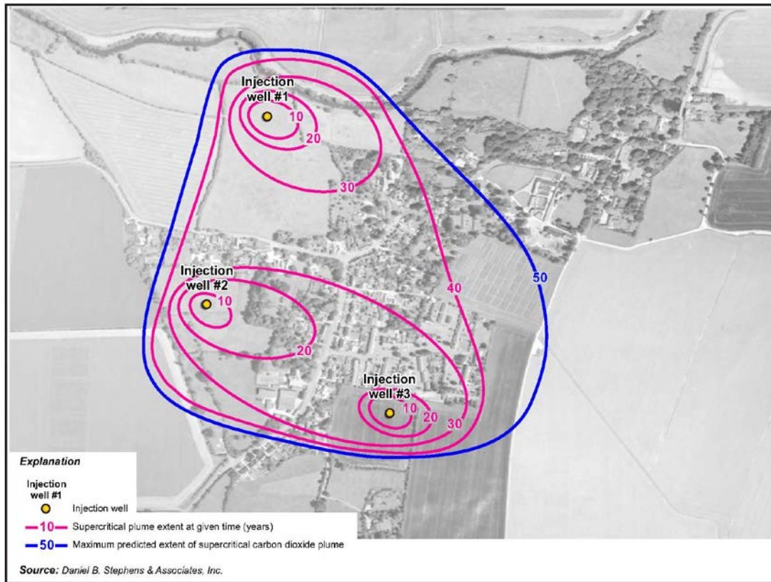
Figure 3-5: Hypothetical Geologic Sequestration Site: Model Predicted Extent of Supercritical Carbon Dioxide Plume Over Time.
